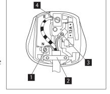
The wire coloured blue must be connected to the terminal «N» or coloured black.
